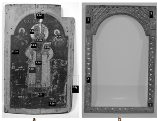
Fig. 1. Sampling points for Saint Nicholas icon: a - frontal side; b - frame
